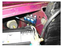
I used Hella relays incorporating a blade fuse to simplify the wiring, and negating the need for inline fuse holders. Utilising a connector with the same three male connectors as a headlamp I could use the original power to the headlamps to control the relays.
